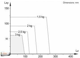
The KR 3 R540 is designed for a rated payload of 2 kg in order to optimize the dynamic performance of the robot. With reduced load center distances and favorable supplementary loads, a maximum payload of up to 3 kg can be mounted. The specific KUKA Load case must be verified using KUKA. For further consultation, please contact KUKA Service.
